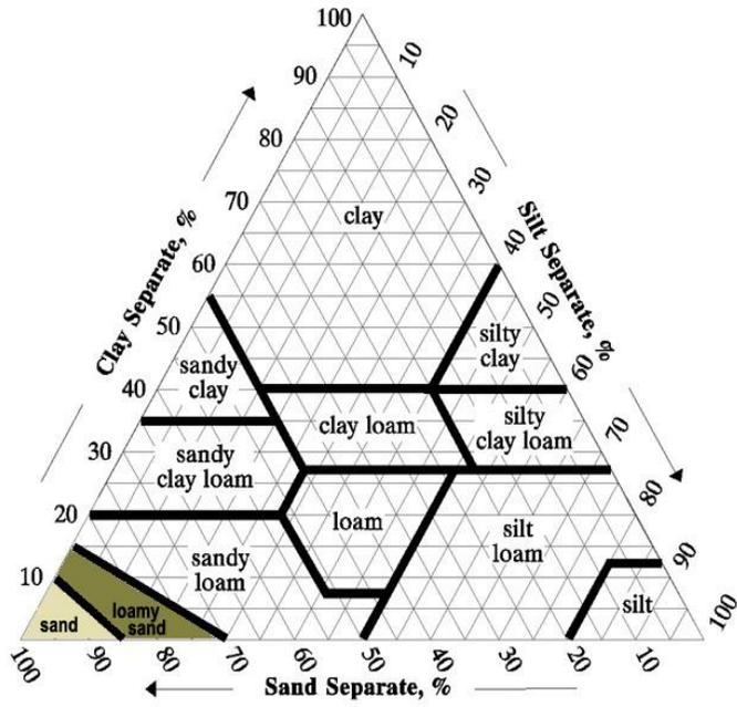
**Figure 5-** The Soil Texture Triangle (US Geological Survey) was used to classify the sediment on Sedge Island using the composition fractions found.
