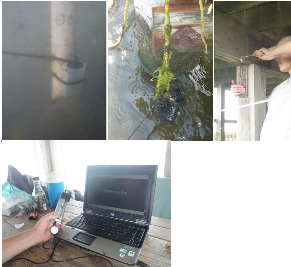
Figure 6. HOBOb® pendant 1 fastened to clam bed pole (Top-left). HOBOb® pendant 2 tied in black zip bag (Top-middle). TidbiT® being installed into north deck of the Sedge House (Top-right). Uploading data from HOBOb® device (Bottom).
